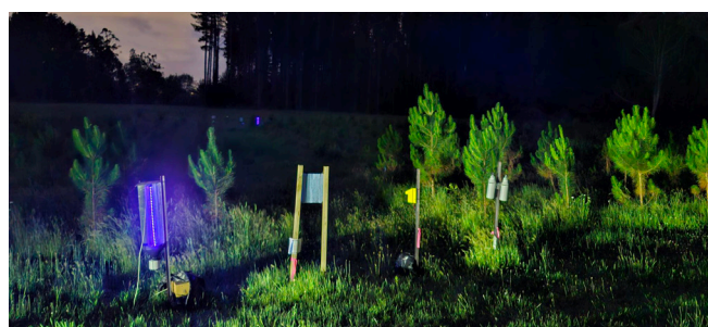
Testing four eDNA collection methods for detecting pests and pathogens: UV light trap, Chux® cloth, battery-powered fan, modified Wilson and Cook sampler.
