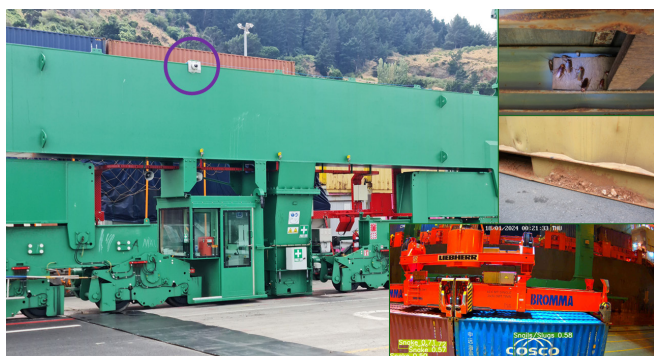
Port container crane with camera (circled), cockroaches on the underside of sea container (top right), soil contaminant on container rail (middle right bottom right), and image of sea container where the AI neural network has classified potential biosecurity risk on a sea container arriving at a port.
