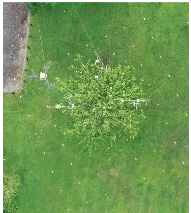
Aerial view of the UAV, the three sampling towers holding samplers at different heights and location within the canopy, and the ground grid layout as the ginkgo tree is sprayed.
